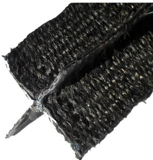
**Set to weave the + (plus) profile directly, the world's first 3D-weaving machine wove it flawlessly to open a new chapter in more than 5000 years of weaving history.**
